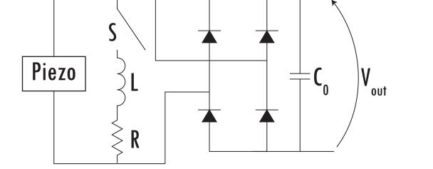
• Flips the charge on the piezo beam at the extreme points of travel. However a rectifier is still required to extract power [1].
