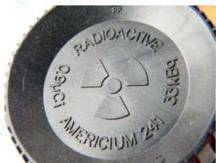
Smoke Detectors using Am-241 as ionizing source
