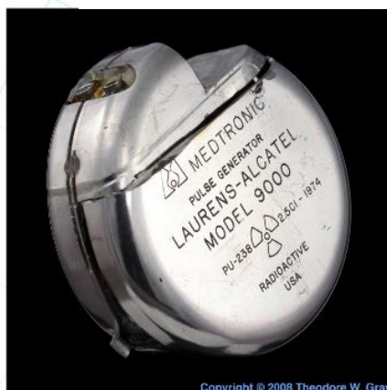
Pacemaker powered by Pu-238 decay (1974)
