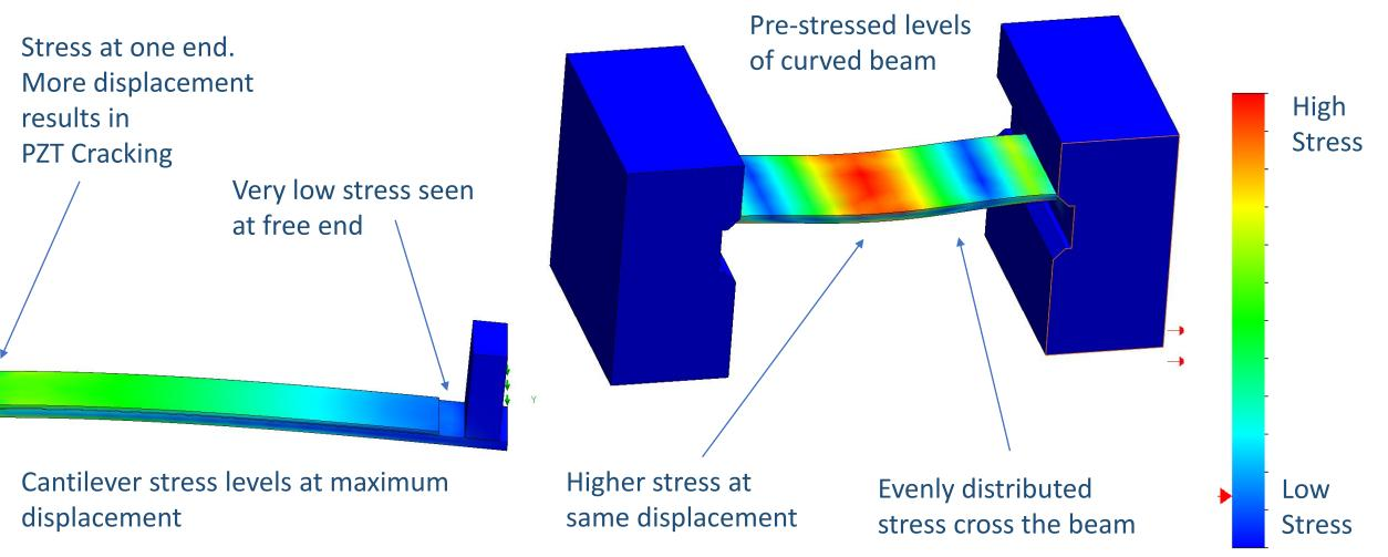
A force is applied to the centre to the outer curved face to induce a "Snap-Through-Action" (STA) of the beam. The beam is then sat in a negative curvature state and is excited from the other face again. The input frequency, maximum displacement, and resistive loads were varied in a set of early stage experimental tests. These illustrations demonstrate the differences in stress areas in a PZT beam.
