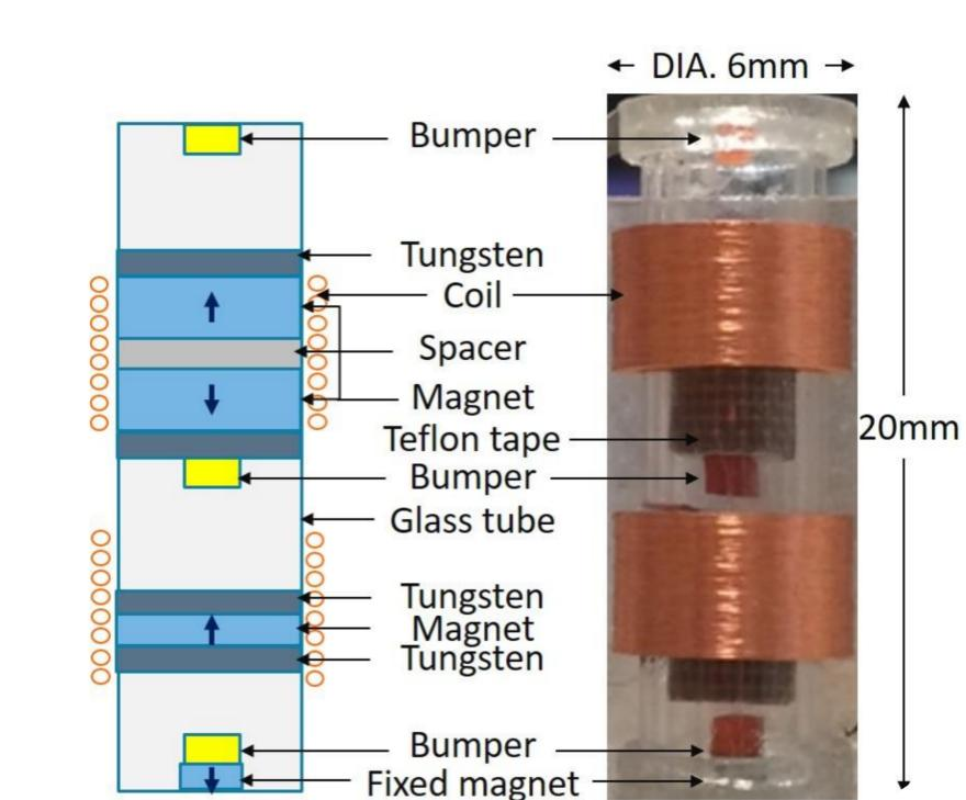
for the 0.5 mm movable bottom mass. The weight of movable masses are 1.52 grams and 0.59 grams for the top mass and the bottom mass, respectively. The coil fill factor is 0.54. Crepe rubber bumpers are added to conserve kinetic
