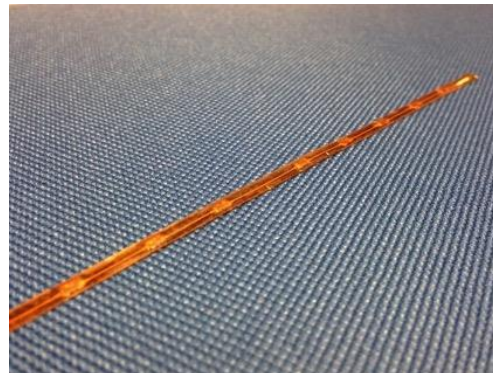
Test circuit with encapsulating moulded Kapton top layer
