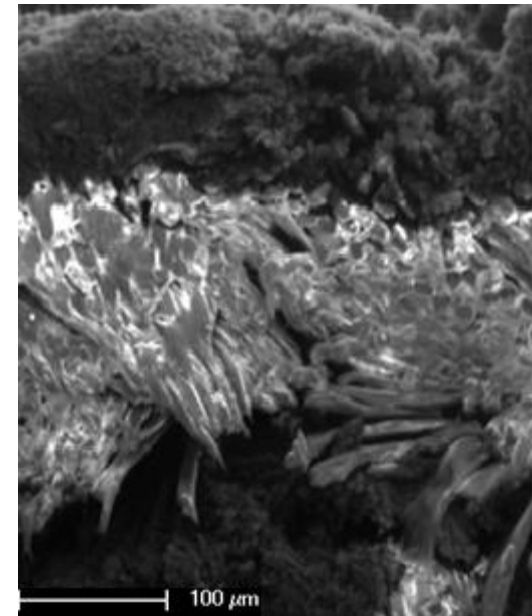
Controlled spraying leaves center of textile uncoated
